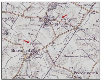
Left Ordnance Survey map of 1901-1902. Shown Sharnford's windmill and Sapcote's derelict tower windmill. mill Sapcote's situated on the Leicester road, built in 1806 on the site of an old former windmill. It was constructed of red brick at a cost of £1300 2s. 3d. The money for this construction work was raised by subscription with investors receiving
