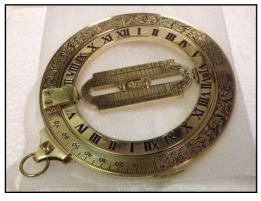
A two-ring universal equinoctial ring dial - was a cutting edge scientific instrument in its time, which is about 500 years ago! Essentially it is a type of sundial that allows you to tell the time wherever you are, so long as the sun is shining.
